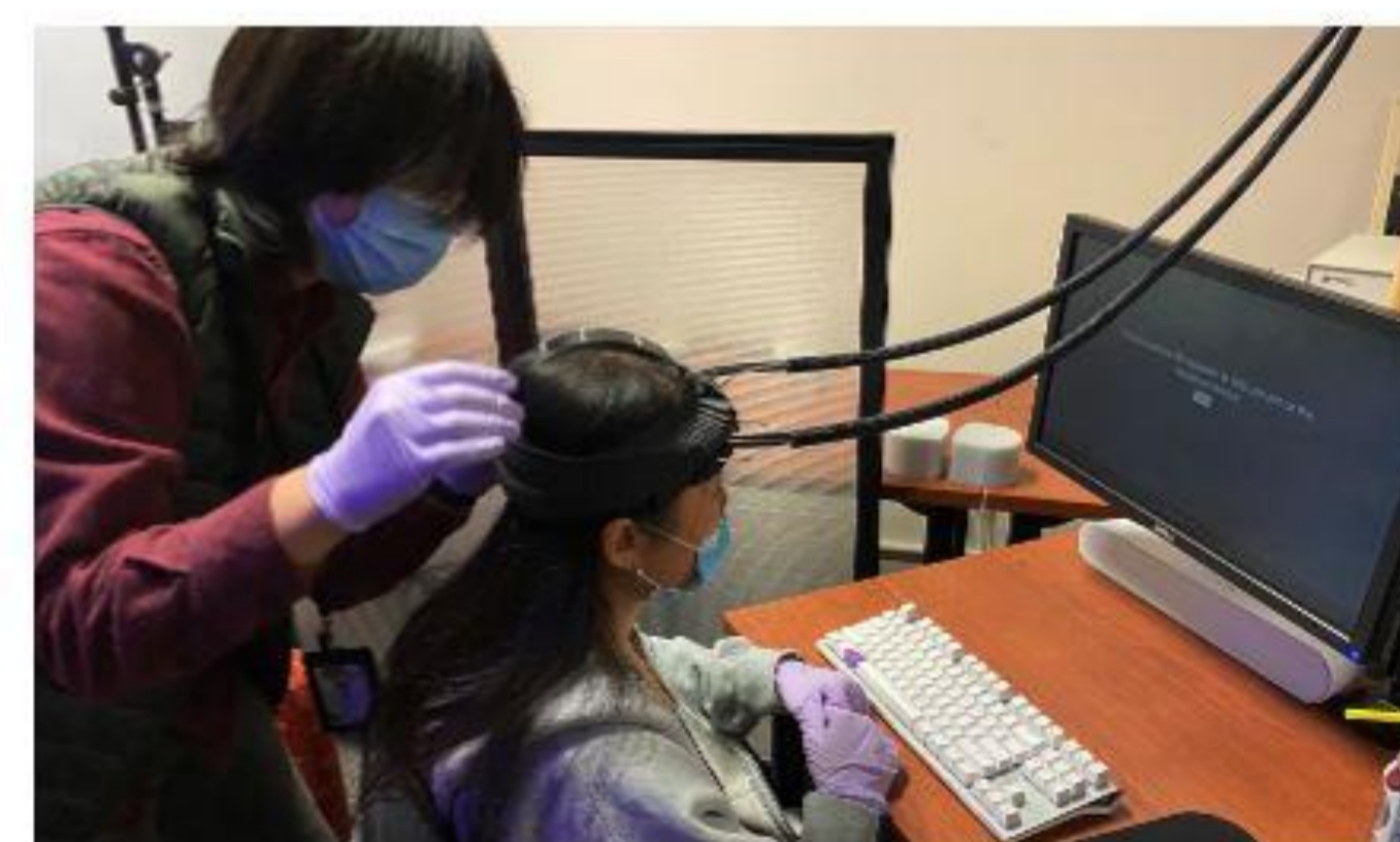
(a) A subject wearing the fNIRS headband, placed by the operator before each experiment began.
